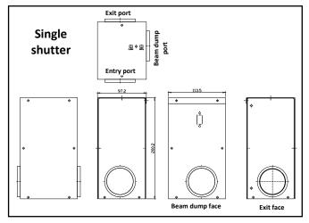
The dual shutter enclosure measures 238mm long compared to the single shutter which is 113.5mm long
