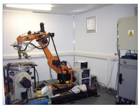
Inside view showing robot mounted laser and laser-safe air vents
