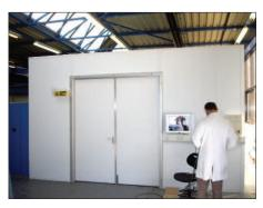
Laser enclosure with interlock system and CCTV
