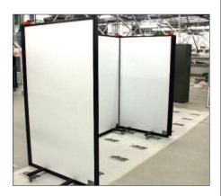
The screens consist of a 50 mm thick sandwich of steel and a special lightweight laser-blocking material, with a white laminate finish on both sides. This is mounted on a powder-coated steel framework, with heavy-duty lockable castors.
