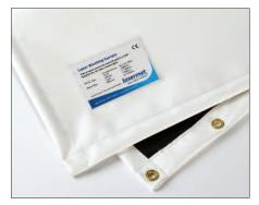
The material is fireproof. When irradiated with greater than 0.5 MW/m² it will emit a non-hazardous smoke and may glow, thus indicating that a stray beam is present. Protection times given by the material at various power densities are shown in the specifications below.
